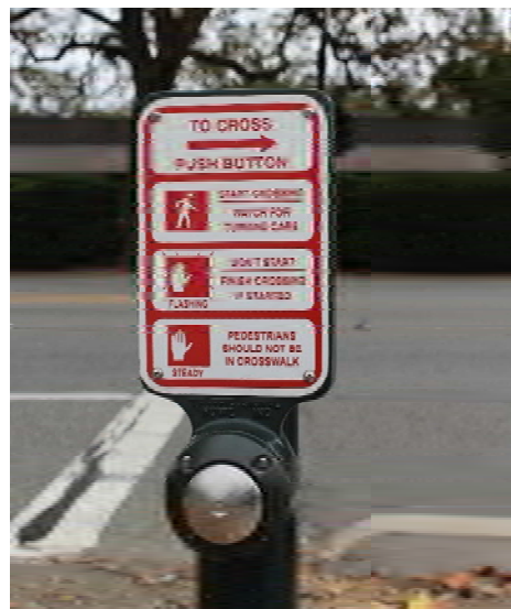
A pedestrian push-button provides information on when pedestrians should cross.
